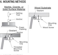
• Apply a generous bead of silicone sealant into the groove around the perimeter of lavatory to
