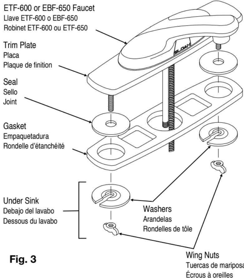
The ETF-578-A Trim Plate Kit contains all of the components necessary to adapt an ETF-600 or EBF-650 sensor-activated lavatory faucet to a sink with 8" spread holes.
