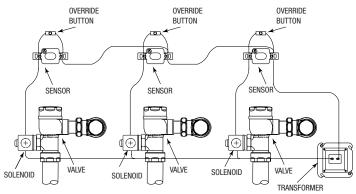
**NOTE:** One Transformer serves up to ten (10) OPTIMA Closet/Urinal Flushometers. Specify number of transformers required accordingly.
