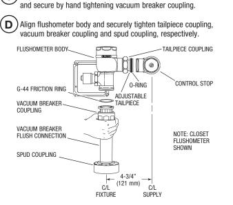
Align flushometer body on top of vacuum breaker flush connection
