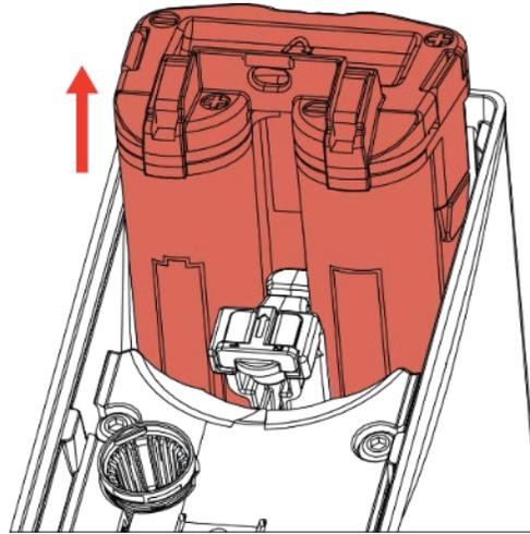
The self-contained battery pack lifts out. Uses 4 common, inexpensive, off-the-shelf, AA alkaline batteries.
