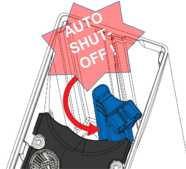
Rotating the solenoid turns off the water! No need to access control stops below deck!
