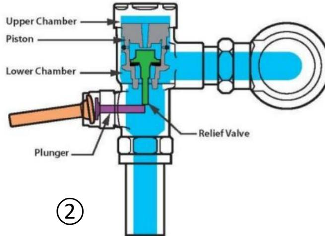
Moving the handle causes the piston to slide up, releasing water into the fixture
