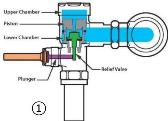
Incoming pressure to the upper chamber seals the piston down over the main seat
