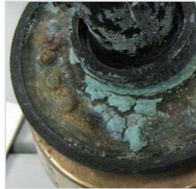
Debris blocking diaphragm bypass
