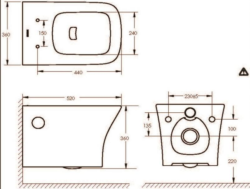
**Note:-**All vitreous china dimensions shown in these drawings are nominal. Dimensions can vary within the tolerances established in the governing BIS standard. Please take this into consideration when planning rough-in and plumbing layouts. Product illustrations shown are representative only; actual products may vary. Sloan reserves the right to make changes in product characteristics, packaging or availability at any time without notice.
