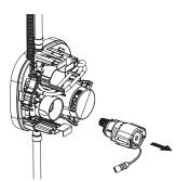
Insert solenoid caddy assembly into control module lining up arrows. Turn solenoid caddy assembly clockwise 45°.
