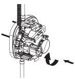
Remove filter from solenoid caddy assembly.
