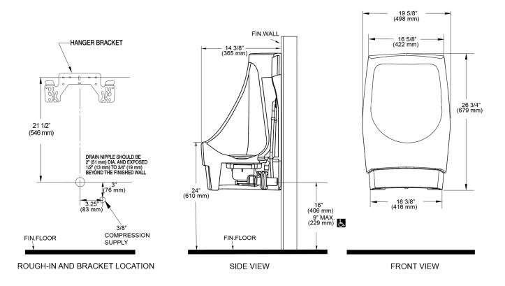
NOTE: ADA urinal rim height requirements allow all heights 17" and below. Sloan strongly recommends roughing in the drain to achieve a 16<sup>1</sup>/<sub>2</sub>" rim height or less to ensure compliance.
