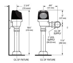
NOTE: All vitreous china dimensions shown in these drawings are nominal. Dimensions can vary within the tolerances established in the governing ASME A112.19.2/CSA B45.1 standard. Please take this into consideration when planning rough-in and plumbing layouts.
