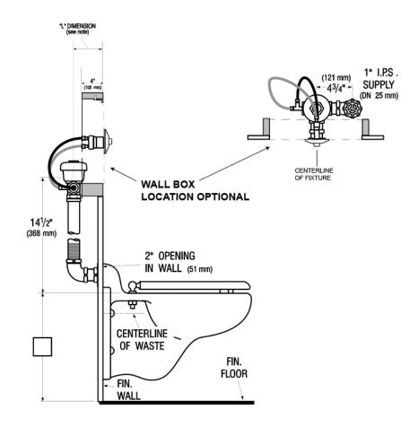
NOTE: "L" Dimension is the Wall Thickness (to the nearest whole inch) plus 2<sup>3</sup>/<sub>4</sub>". Specify "L" Dimension when ordering Flushometer.
